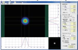
This is an example of using a light source of 1550 nm and observing an infrared beam spot of about 10  $\mu m\phi$  collected by the light collection module.
