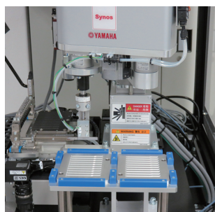
*Sample transfer robot and sample tray for individual pieces sample
